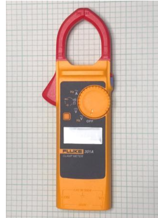
Fluke 301A Clamp Meter (Photo by Norbert Doerry CC BY 4.0)
